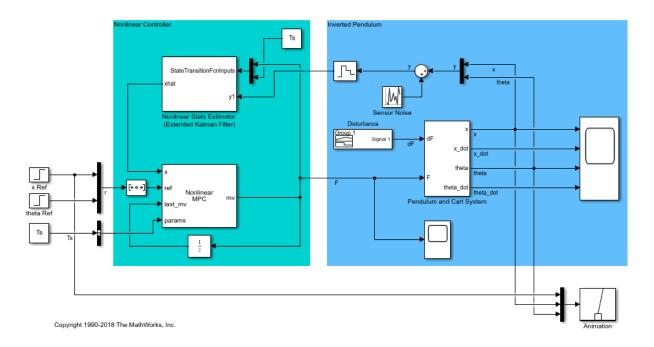
In this model, the Nonlinear MPC Controller block is configured to use the controller nlobj.
